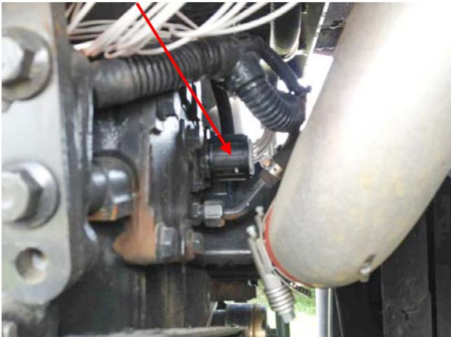
**3)** Plug the male connector from the Ag Diesel Solutions module into the stock location on the engine head. Align the inside section of the connector to the stock plug and then rotate the outer shell clockwise to tighten.
