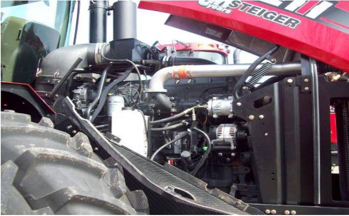
**2)** Unplug the stock injector connector from the front side of the engine head. To loosen, rotate the outer shell of the connector counter-clockwise.
